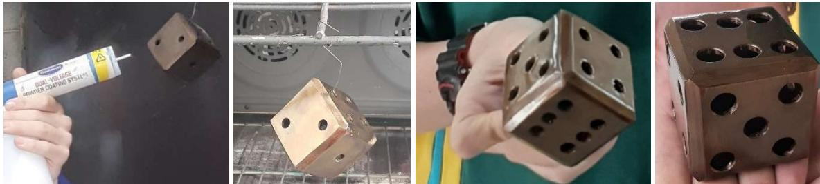
Once ground, the dice is drilled, sprayed with powder coating & oven baked. We use a clear powder coating, which combined with a heat induced colour change of the metal to provide the final colour.
