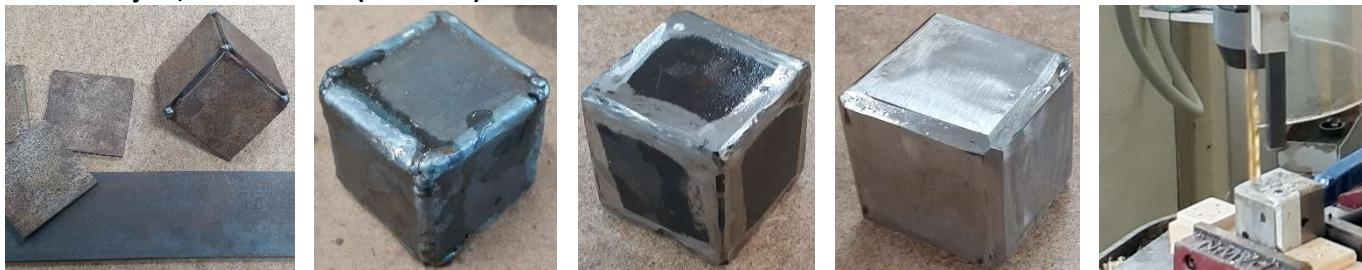
Starting with a length of 50x3mm flat steel bar, students cut these to length, tack weld them in a jig to assist with alignment, then weld the whole dice. The welds are then ground flat, which hides some imperfections, but exposes others such as voids that need to be re-welded and ground.
